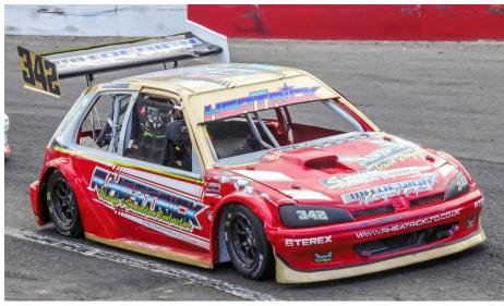
**A.** Any four-seater, front-engined, saloon or hatchback, constructed of steel, the overall length must not exceed 3988mm (157") and the overall width must not exceed 1702mm (67") when ready to race. Consideration will be given to any modern vehicle which falls outside these specified measurements in its original form, but can comply when prepared for racing, as follows: **Length**: By reducing the depth of either the front or rear bumper.
