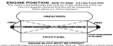
The centre crankshaft pulley bolt must be on the centre-line of the car. There will be a ± 25mm tolerance. NB: Both Wings must be the same width (i.e. no offset panels).
